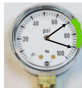
Correct dynamic pressure, before, during, after pour
